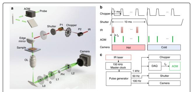
**Fig. 2 Scheme of the BSTP microscope. a** Illustration of the BSTP microscope. A common-path diffraction phase microscope was built on an inverted microscope, and an IR beam was introduced for BSTP imaging. AOM: acousto-optical modulator. P1, P2: gold parabolic mirrors. OL: objective lens. L0, L1, L2: lenses. G: grating. PH: pinhole. **b** Timing diagram.  $t_d$ : delay of the probe pulse relative to the start of the IR pulses in each burst. **c** Clock hierarchy.
