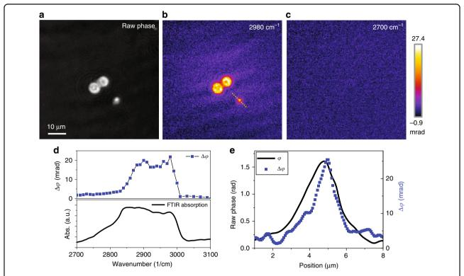
**Fig. 4 BSTP imaging of polyurethane beads. a** Quantitative phase image of PU beads. **b,c** BSTP imaging of PU beads at an absorption peak of 2980 cm<sup>-1</sup> and an off-resonance peak at 2700 cm<sup>-1</sup>, respectively. **d** BSTP spectral profile of PU beads (top) and the measured standard FTIR spectrum (bottom). **e** BSTP (blue squares) and raw phase (black line) profiles of the smaller PU bead across the dashed line marked in **b**.
