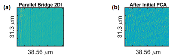
Fig. 6. Parallel defect image with 2^{nd} order difference. (a) Before and (b) after PCA.
