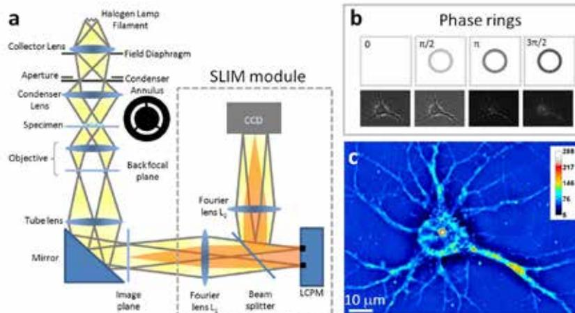
Figure 8. SLIM principle. (a) Schematic setup for SLIM. The SLIM module is attached to a commercial phase contrast microscope (b) The phase rings and their corresponding images recorded by the CCD. (c) SLIM quantitative phase image of a hippocampal neuron.
