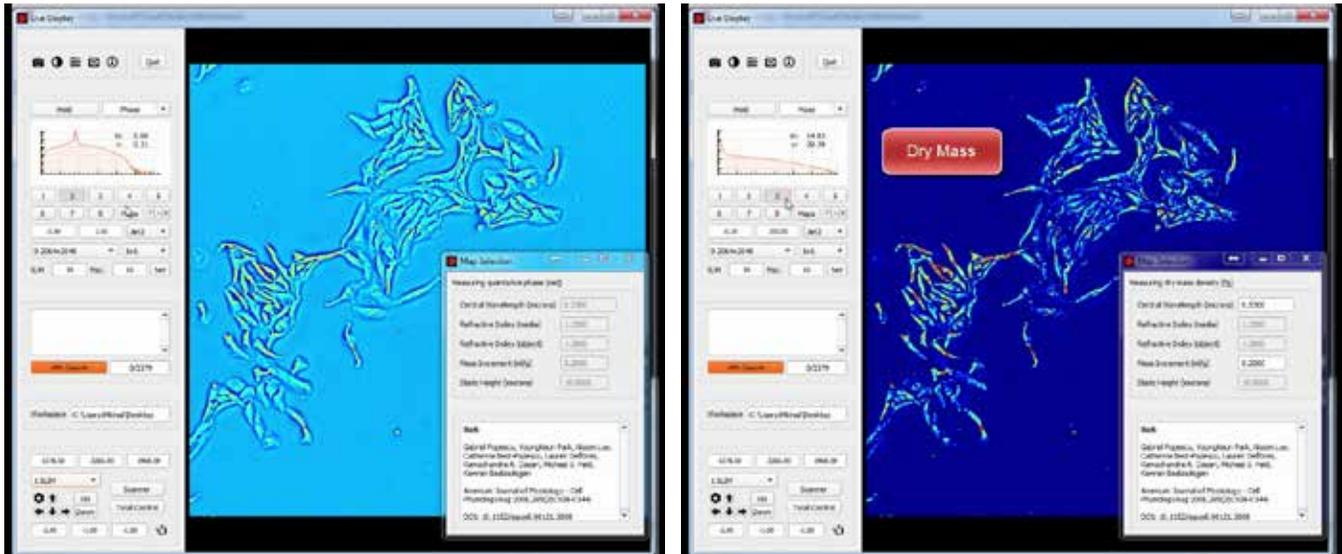
Figure 1. CellVista software working in phase measurement mode (measurement in radians) and in dry mass measurement mode (measurement in picograms). The setting can be changed in the Map Selection menu.
