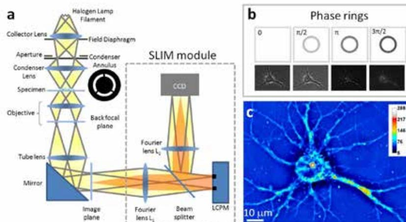
Figure 7. SLIM principle. (a) Schematic setup for SLIM. The SLIM module is attached to a commercial phase contrast microscope (b) The phase rings and their corresponding images recorded by the CCD. (c) SLIM quantitative phase image of a hippocampal neuron.
