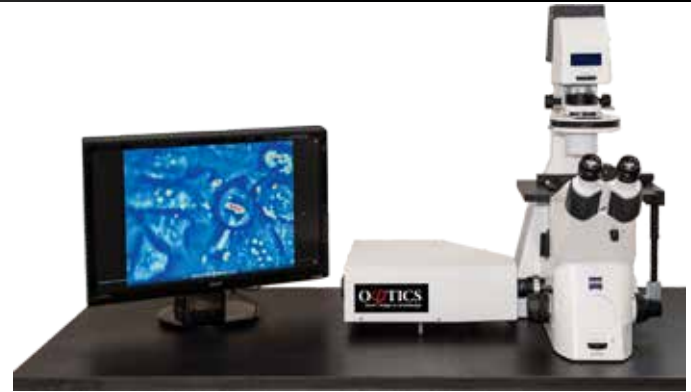
Figure 9. Phi Optics SLIM module attached to a ZEISS Axio Observer Z1 microscope
