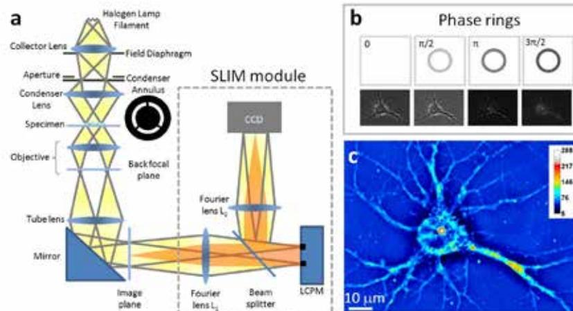
Figure 9. SLIM principle. (a) Schematic setup for SLIM. The SLIM module is attached to a commercial phase contrast microscope (b) The phase rings and their corresponding images recorded by the CCD. (c) SLIM quantitative phase image of a hippocampal neuron.
