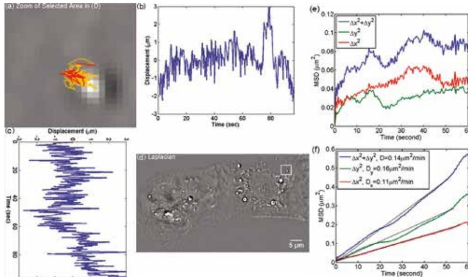
Figure 4. MSD measurement for particles within the cardiac myocytes in Fig. 2. (a) Zoom into the selected area shown in (d); (b) Displacement in Y direction; (c) Displacement in X direction. (d) Laplacian of the phase map; (e) MSD for the particle shown in (a). (f) MSD ensemble-averaged over 15 particles in (d). [2]
