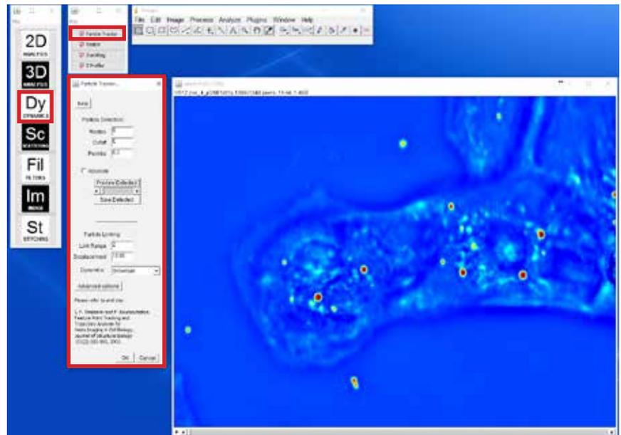
Figure 2. Particle tracker parameter setup window and a SLIM phase map of a heart cell containing particle-like organelles.
